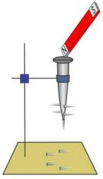
When the magnet is removed from the head of the nail, the pins fall down showing demagnetism.
