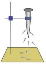
The property by which an ordinary piece of iron acquires magnetic properties due to the presence of another magnet it is called magnetic induction.
