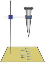
When a magnet is touched to the head of the nail, some pins at the base of the stand cling to the nail. This is because the nail turns into a magnet and hence requires the properties of magnetism.
