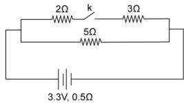
Resistance (R1) of the circuit =  $(5+0.5)\Omega = 5.5\Omega$
