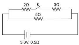
The diagram above shows a circuit with the key k open. Calculate:
