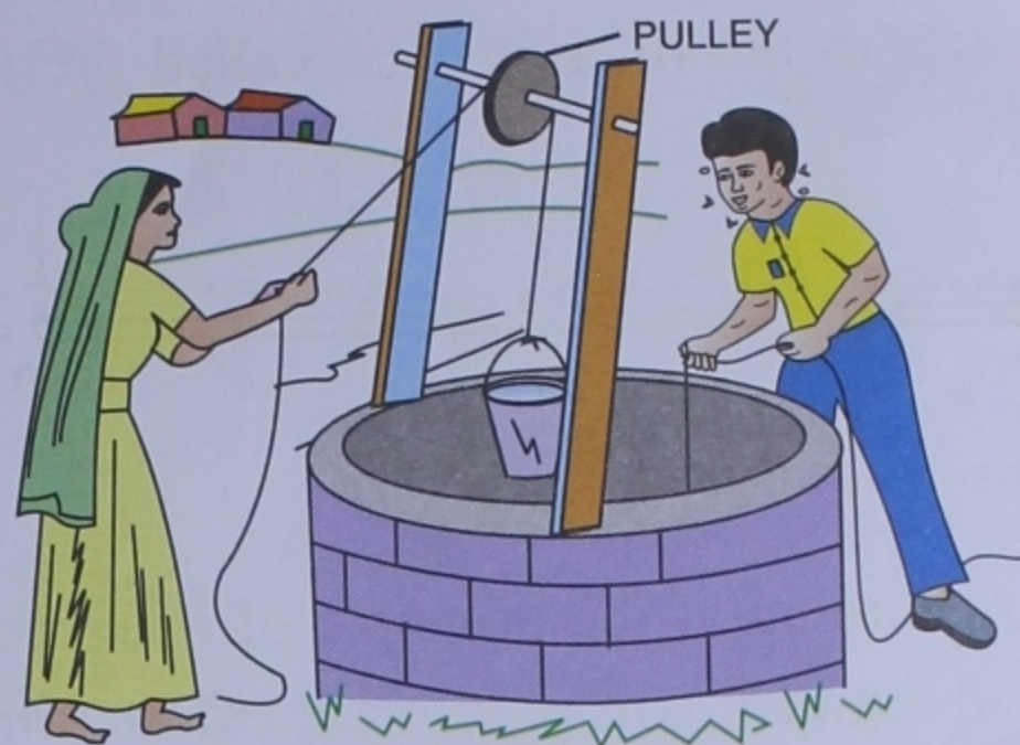
Fig. 6.2 Examples of a pulley being used as a simple machine
