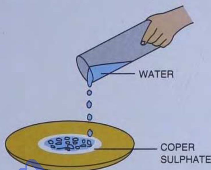
Fig. 5.11: Adding water to white copper sulphate turns them blue
