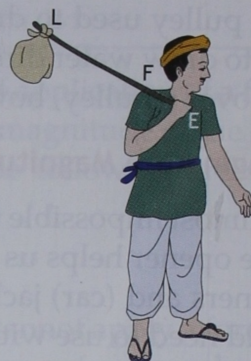
Fig. 5.6 The basic parts of a lever
