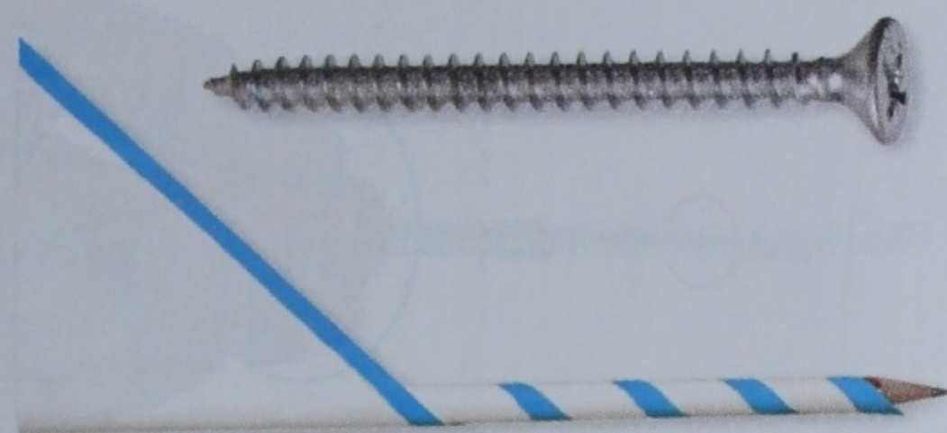
Fig. 5.13 A screw is a nail with an inclined plane wrapped around it.
