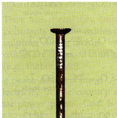
Fig. 4.2 Rust on a nail
