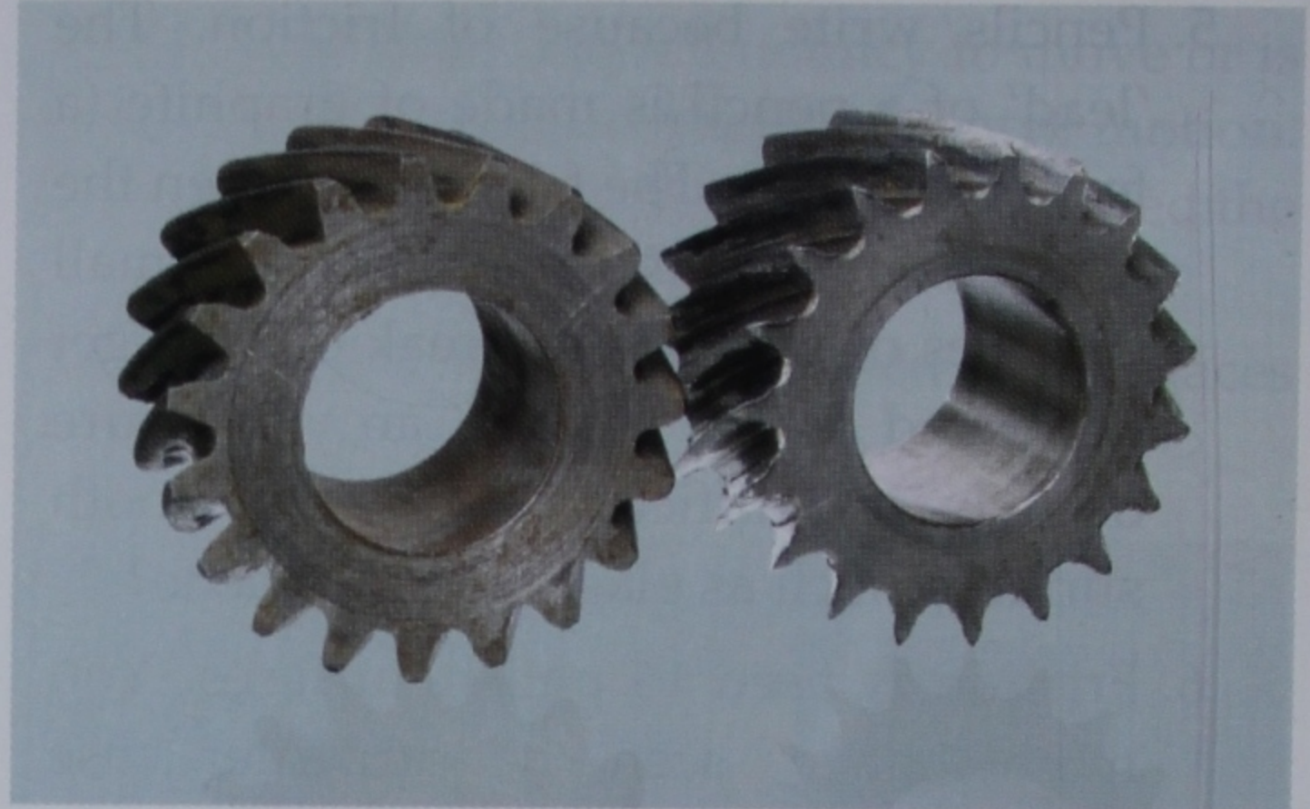
Fig. 3.10 The teeth of the gear on the right have worn out (become thinner) due to friction.
