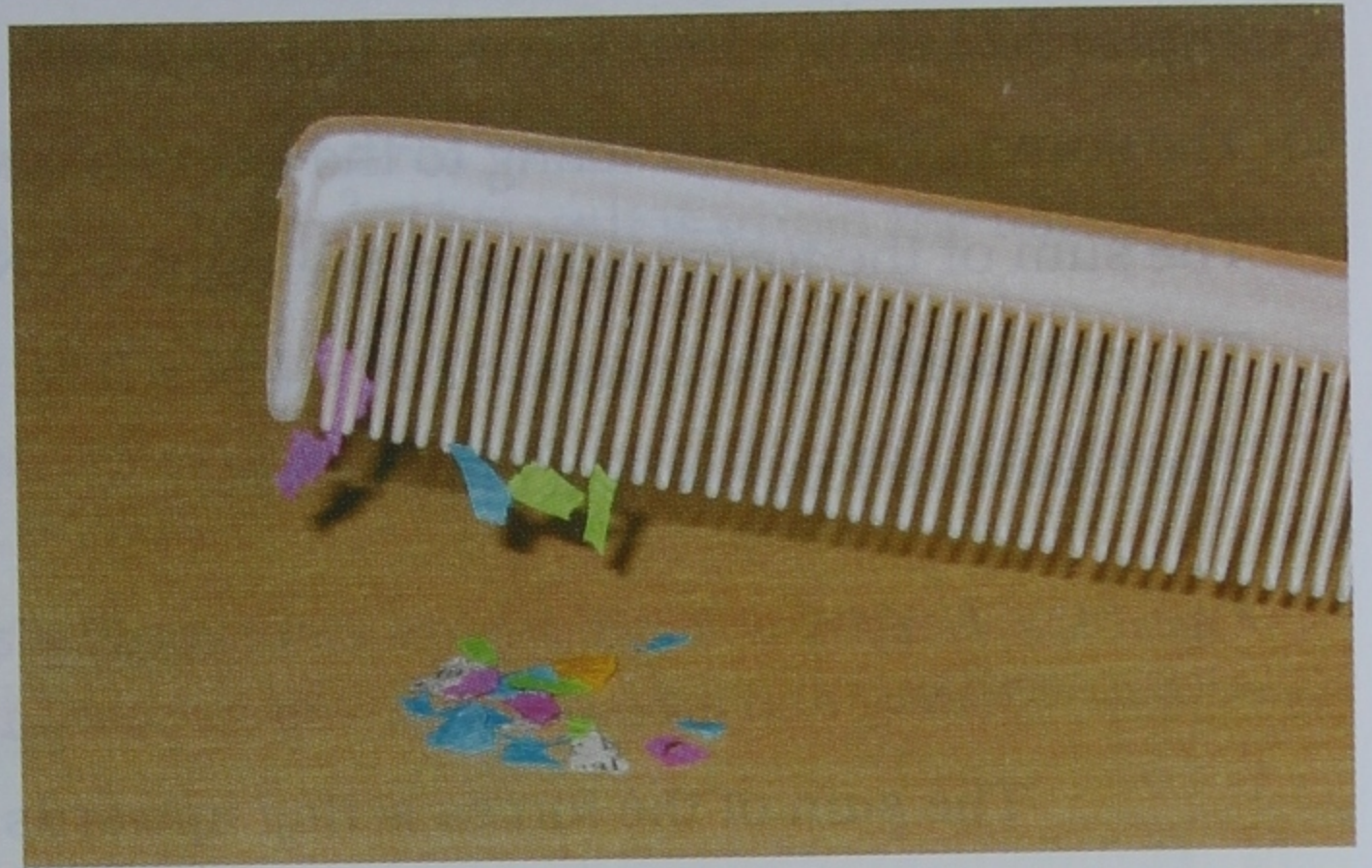
Fig. 3.19 The charged comb attracts the bits of paper from a distance.
