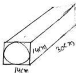
$$\text{Volume of cylinder} = \frac{\pi d^2}{4} \times h$$
