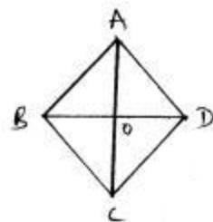
$$\begin{aligned}\text{(i) Area of rhombus} &= \frac{1}{2} \times (\text{product of diagonals}) \\ &= \frac{1}{2} \times (13 \times 5)\end{aligned}$$
