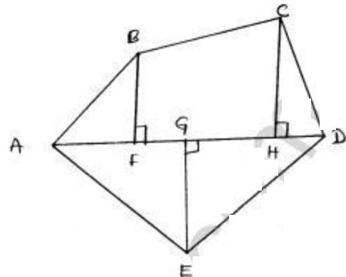
$$\begin{aligned} \text{Area of polygon } ABCDE &= \text{Area of } \triangle ABF + \text{Area of } \triangle BCF + \text{Area of } \triangle CHD \\ &\quad + \cancel{\text{Area of } \triangle ADE} + \cancel{\text{Area of } \triangle DGE} \\ &= \frac{1}{2}(AF \times BF) + \frac{1}{2}(BF \times CH) \times FH + \frac{1}{2}(DH \times CH) + \\ &\quad \frac{1}{2}(AD \times EG) \end{aligned}$$
