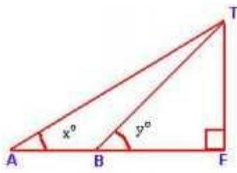
$$\tan x^\circ = \frac{2}{5}, \quad AF = 200\text{m}, \quad AB = 80\text{m}$$
