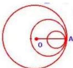
$\therefore$  The locus of the centre of a circle which touches the circle at the fixed point A on it is a line joining the points O and A.
