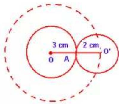
If the circle with 2cm as radius touches the given circle with 3cm as radius internally, then the locus of the centre of the circle will be a concentric circle with radius  $3-2 = 1\text{cm}$ .
